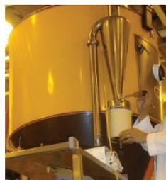
**Method description:** ingredient is atomized via spraying mechanism into a superheated chamber where hot gases cause raw material to instantly dry
